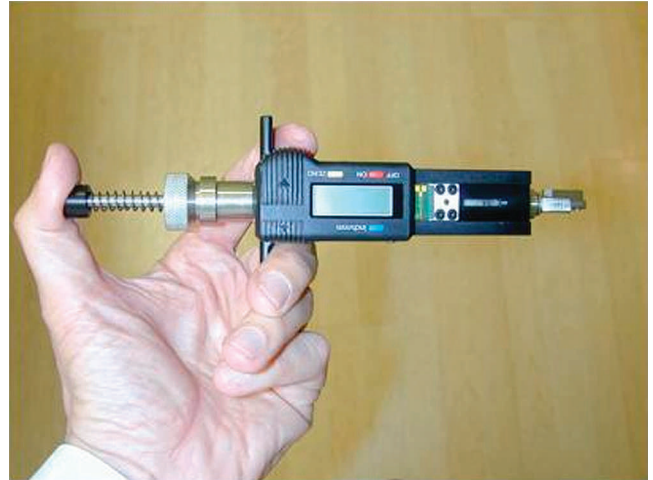
FIG. 10.11. The diameter of the collected hair is calculated to find the trichometric index (TI) (Image courtesy of Bernard Cohen, MD).
